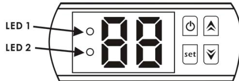
When the heat pump is running, the LED display shows the water inlet temperature.
